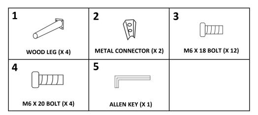
STEP 1: Attach metal connector (2) to backside of seat (B) with bolts (4). using the Allen Key (5).
